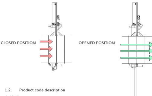
AADA : Medium pressure electro-galvanized sliding damper
