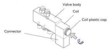
*Step 2*: connect the connector on the coil by sliding it over the three prongs of the coil and lock it in place with the screw on the top of the connector.
