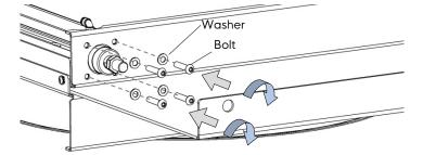
Step 3: Screw the head of the cylinder body to the sliding damper body with washers and bolts.
