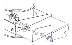
Step 3: Attach the base of the cylinder to the body using nuts, counter-nuts and spacers.
