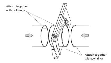
**IMPORTANT**: Make sure to use adequate support on the pipes on either side of the sliding damper to reduce pressure on the sliding damper body and blade.
