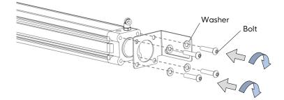
Step 2: Insert the head of the cylinder through the hole in the top of the sliding damper body.
