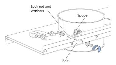
**IMPORTANT**: Make sure that the cylinder is aligned with the body to ensure proper blade movement and avoid premature wear of the components.
