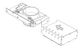
Step 3: Use the bolt unscrewed in Step 1 to attach it to the sliding damper.
