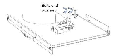
3.3.2 Mounting the coil and connector on the solenoid valve
