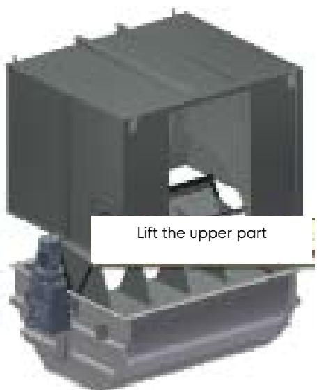
After this, the separation plate can be removed allowing access to the rotor.
