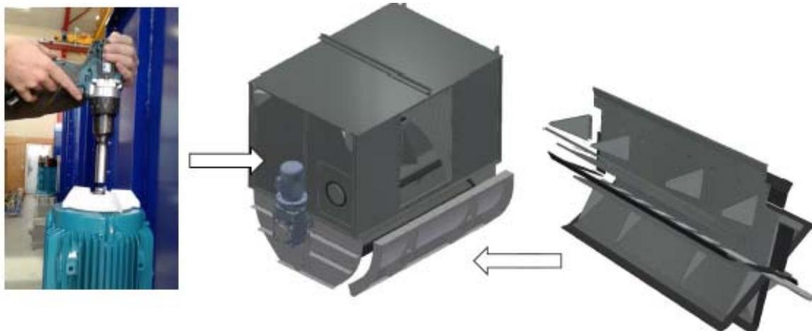
To rotate the rotor, dismount the fan shroud on the motor. This will give access to a bolt on the end of the motor shaft which can be rotated using either a wrench or a non-impact driver.
