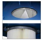
Easy filter replacement performed by bayonet suspension, which is loosened from clean air chamber with limited dust generation and inserted into sack.
