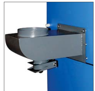
Cleaning tap Built-in flap valve ø76 mm on inlet connection for cleaning around unit af-ter service and dust con-tainer emptying.
