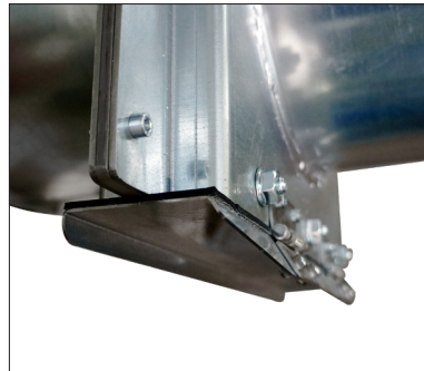
Discharge lid on the underside of the damper
