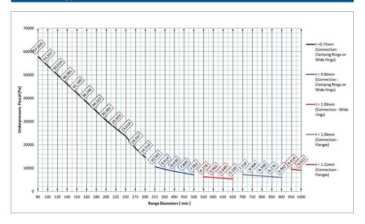
Maximum underpressure chart for standard Formula Air light gauge Sendzimir ducting.
