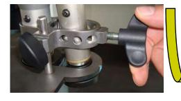
Step 5 : Slide the pipe edge between the two wheels, with the machine battery towards the inside of the pipe, and turn the upper butterfly nut to bring the adjustable wheel against the pipe :
